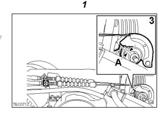
and verify that the gap between the cam and the lever is set between 0.5 - 1.5 mm (0.019 - 0.029 in), dimension 'A' in illustration 1.
